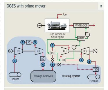
Preheating and reheating (to 200°F) is accomplished by hot water in shell-and-tube heat exchangers (STHX). Circulating water is heated in a separate STHX (WHTR in the diagram) using hot water from the waste heat recovery unit (WHRU) – basically, a combined cycle heat recovery steam generator (HRSG) without evaporator and superheaters.
